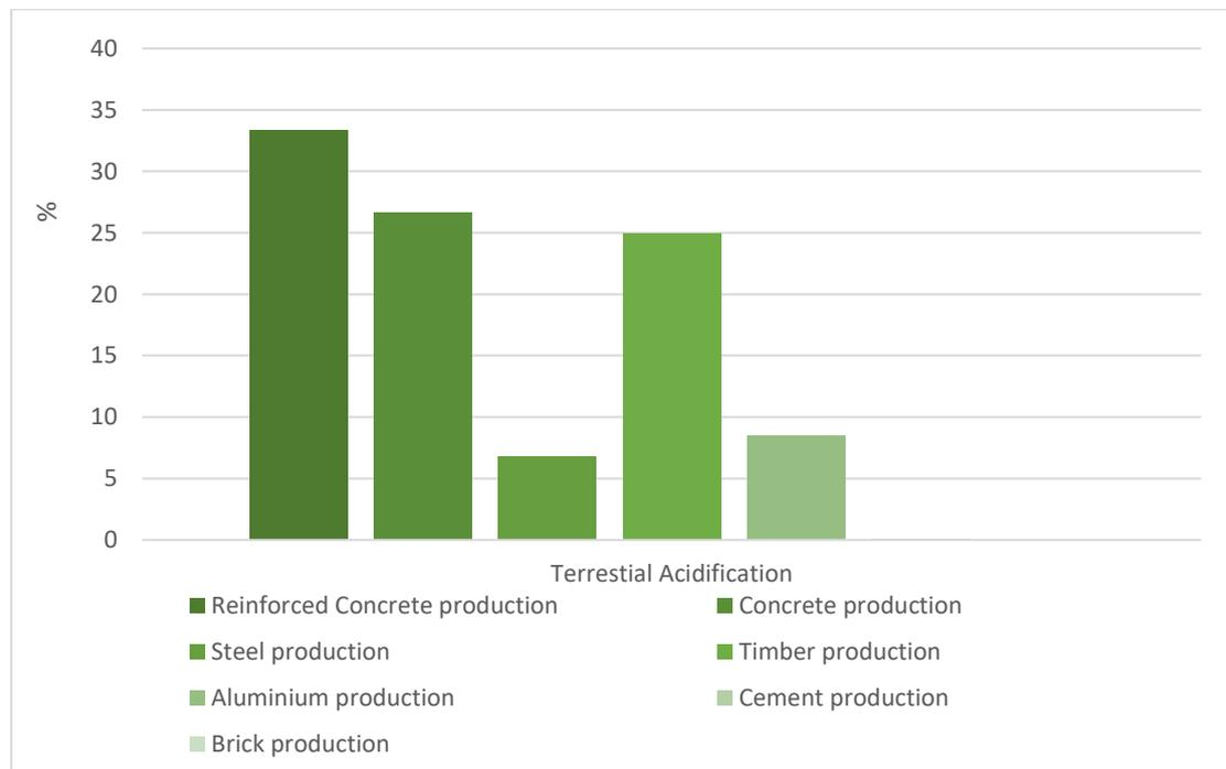
**Figure 5.** % of kg SO<sub>2</sub> emission on the production phase
