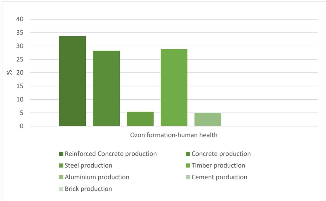
**Figure 9.** % of kg NO<sub>x</sub> on the production phase
