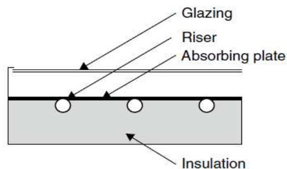
**Figure 12:** Cross section of a basic flat plate solar collector [10]
