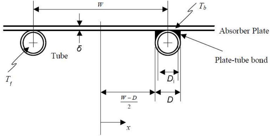
**Figure 15:** Geometric configuration of the absorber plate-tube [23]
