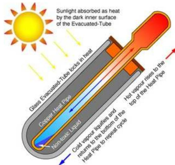
**Figure 9:** Evacuated tube cross section [18]
