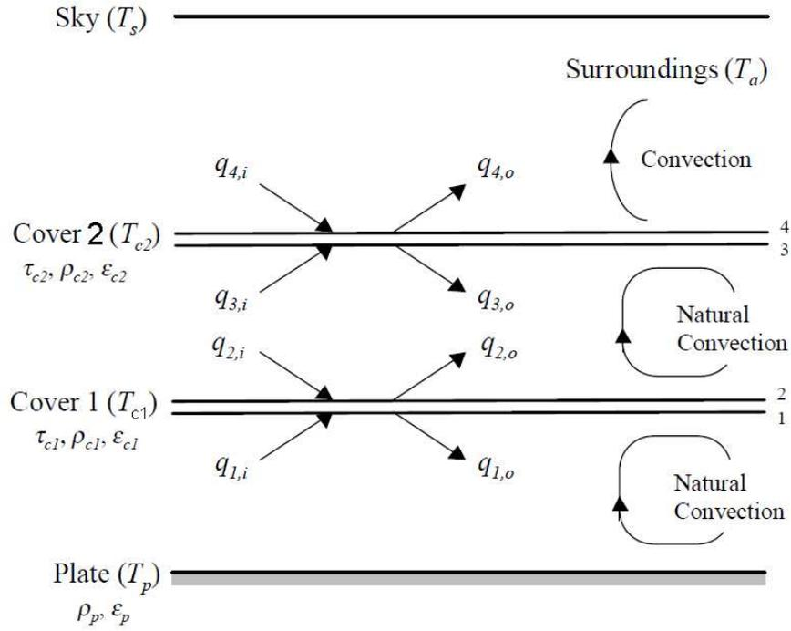
**Figure 14:** Net radiation method for two-cover collector [23]
