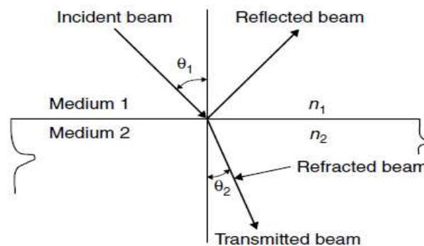
**Figure 13:** Angles of incidence and refraction [10]
