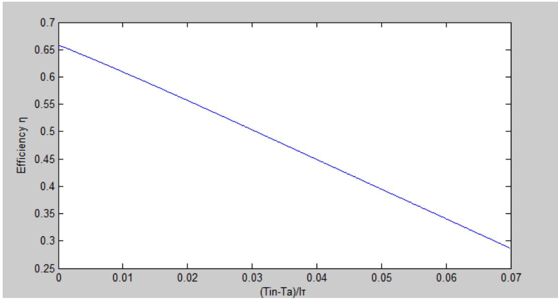
**Figure 17:** Calculated efficiency of collector under test
